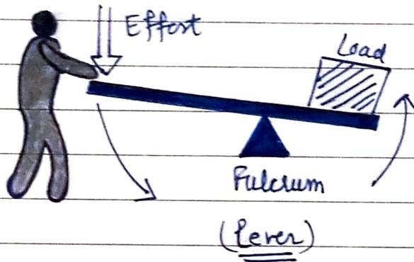
The figure above shows a schematic diagram of a lever. Both the forces, load (L) and effort (E) act on the lever.
