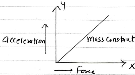
The acceleration produced in a body of constant mass, is directly proportional to force applied.
